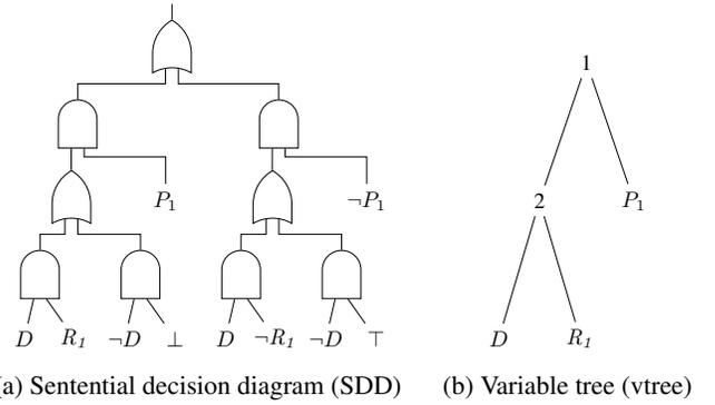
Figure 2: Tractable SDD circuit representation for Sentence 1
